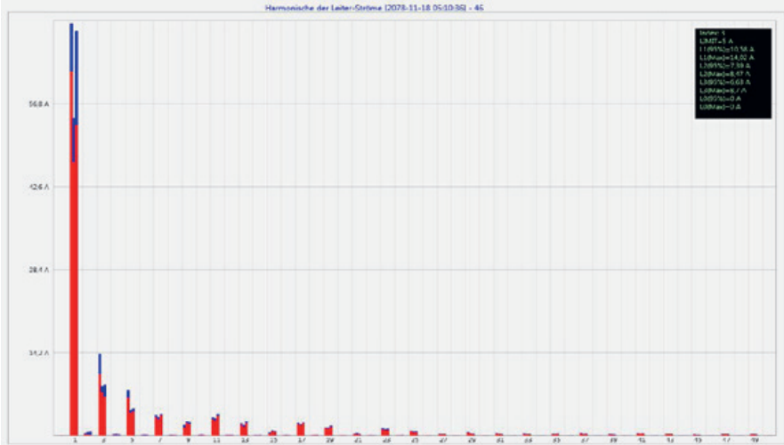
Example: Statistic current harmonics 2nd to 50th - scaling in ampere
